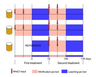
Fig. 2. Experimental design for each soil type: two of the three soil column replicates received the same treatment and one column was used as a reference in the first step of the experiment.
