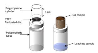
Fig. 1. Soil column devices with an exploded diagram.
