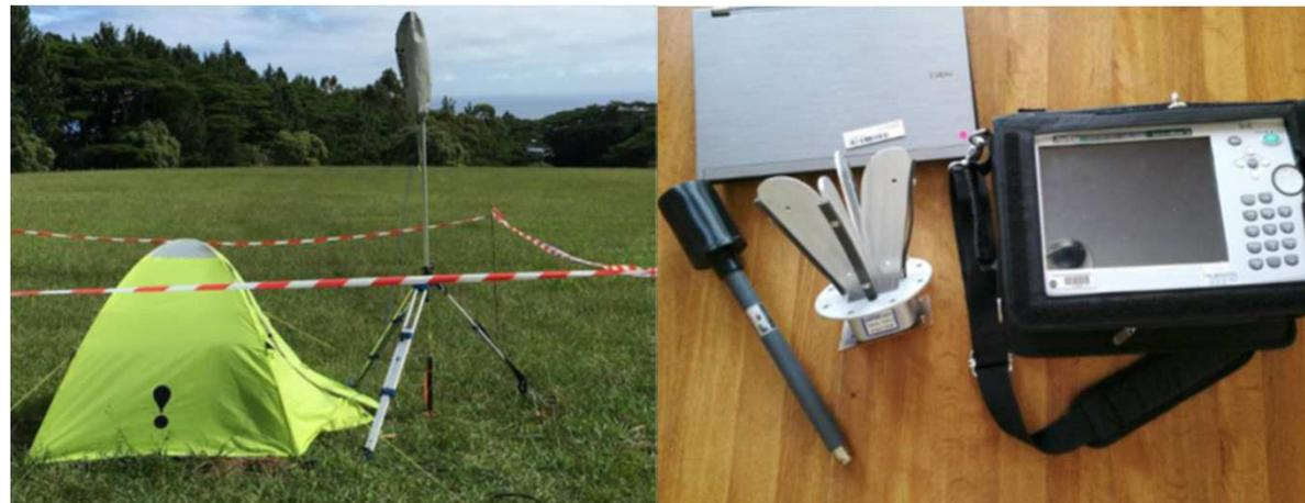
VLBI test equipment with spectrum analyser, 1 to 18 GHz and biconical omnidirectional antenna
