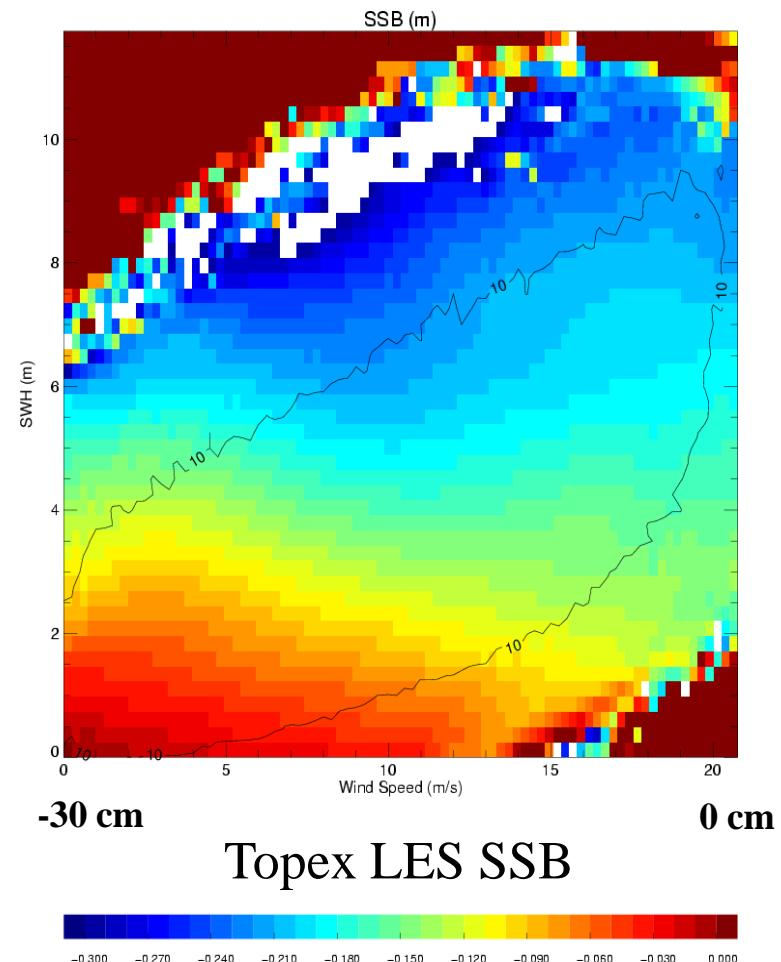
Use of non-parametric methods to estimate SSB (SWH, Wind)
