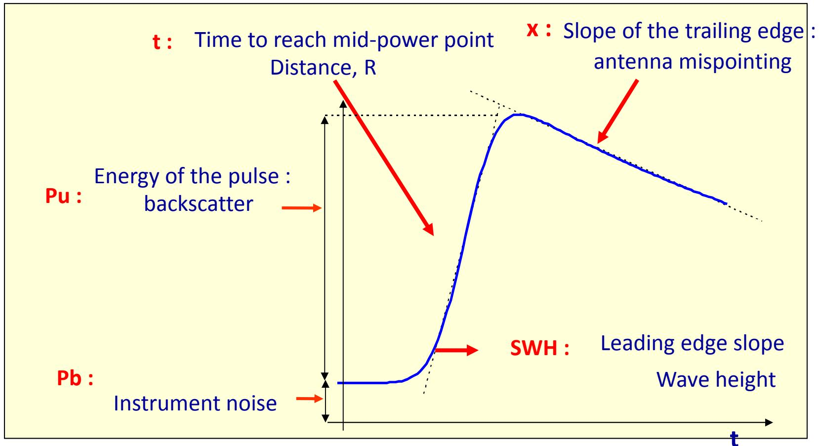
For each averaged waveform (20Hz), fitting procedure between a model and the measured waveform
