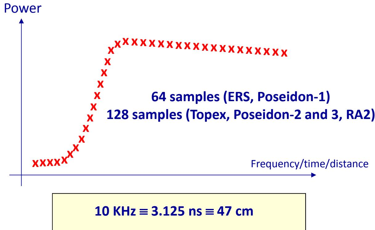
The range resolution of an altimeter is about half a metre (3.125 ns) but the range measurement performance over ocean is about one order of magnitude better. This is achieved by fitting the shape of the echo waveform to a model function which represents the form of the echo (Brown, Hayne) + averaging over a large number of echoes (PRF > 2000 Hz)
