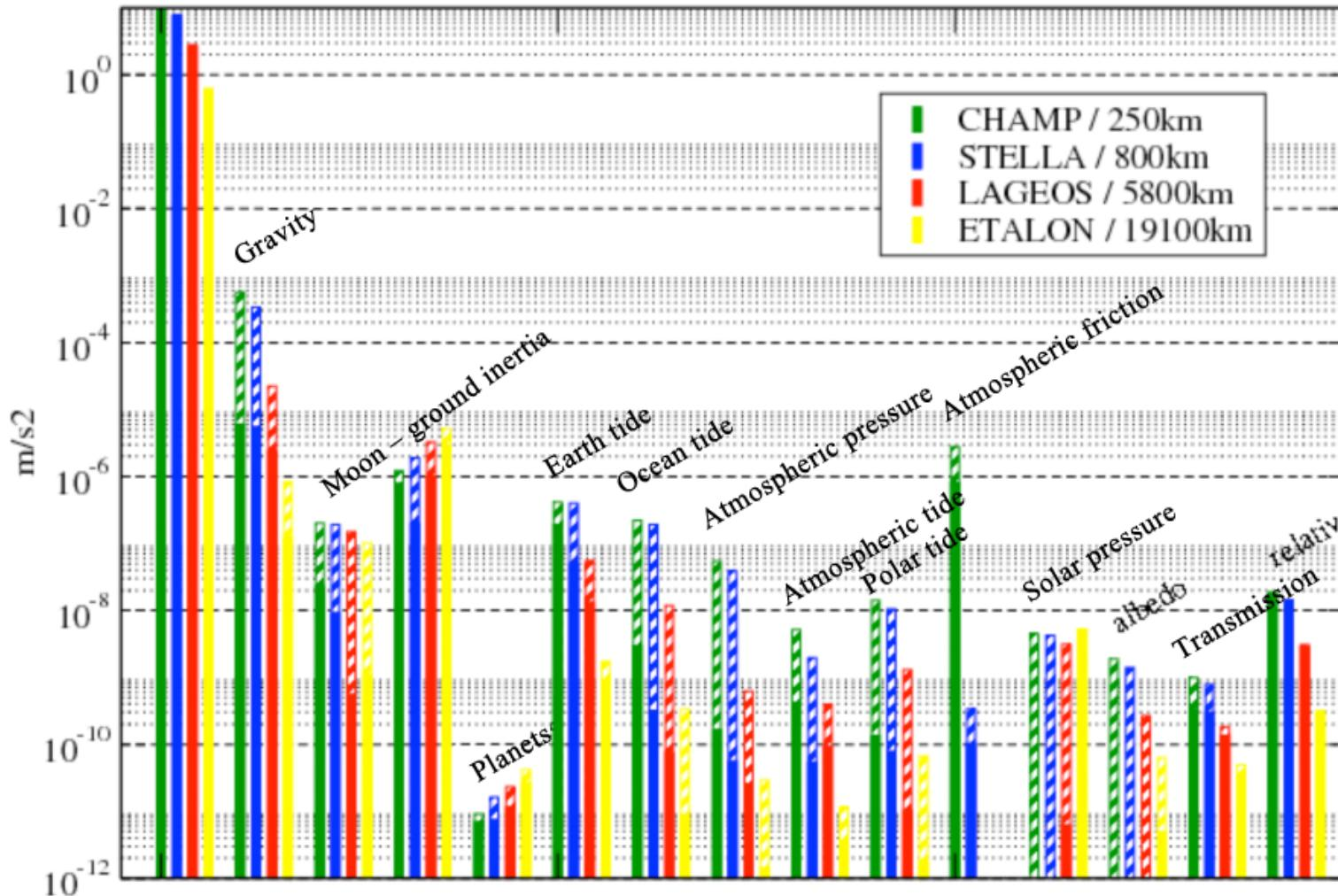
*Some examples of the amplitude of the acceleration taken into consideration for the numerical integration of the movement (the min. and max. values in the course of the arc are entered for each satellite).*
