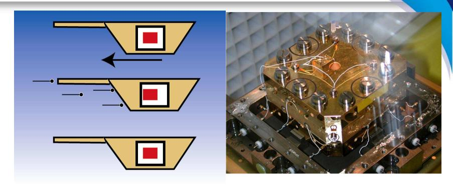
Left: Principles of satellite accelerometry. The motion of a test mass in the shielded interior is measured (kept in place through electrostatic forces). Right: real satellite accelerometer.
