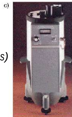
Figure 8. (a) LaCoste and Romberg Model G land gravity meter; (b) Worden Master land gravity meter; (c) W. Sodin T410 land gravity meter; (d) GWR cryogenic gravity meter; (e) Bell BGM5 marine gravity meter; (f) Micro-G Solutions FG-5 absolute drop gravity meter; (g) LaCoste and Romberg borehole gravity meter; (h) LaCoste and Romberg Model S air-sea gravity meter; (i) Scintrex CG-3 land gravity meter.
