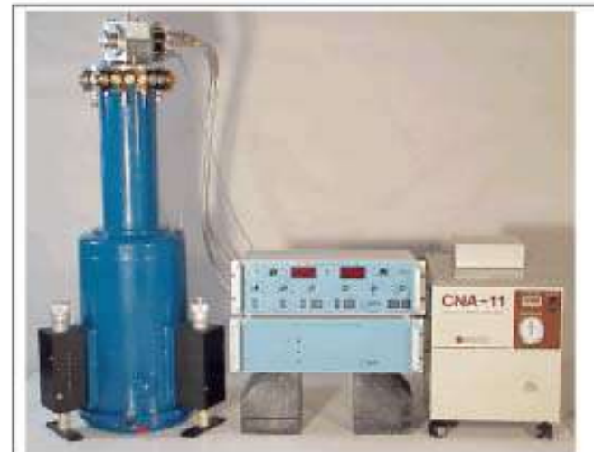
Figure 5: SG operating in a small Dewar using a Sumitomo SRDK-101 coldhead and a Sumitomo CA-11C compressor. Dewar is 10 inches in diameter and 36 inches tall
