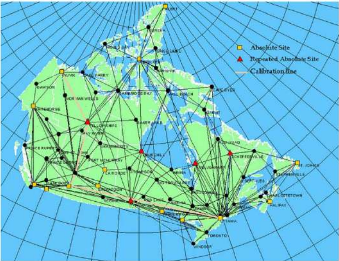
Figure 1. The Canadian Gravity Standardization Network (CGSN). Black lines indicate gravity ties. Yellow squares show sites that have been observed with absolute gravimeters, and red triangles depict sites with repeated absolute gravity measurements.
