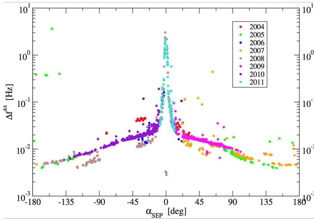
✓ Interplanetary plasma (+ Earth ionosphere) Doppler effect from dual-frequency X/S band on Mars Express.
