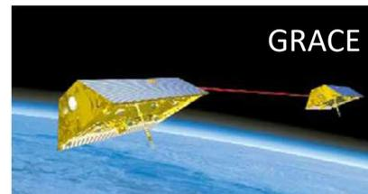
*GPS + SLR + KBR + accelerometer*
