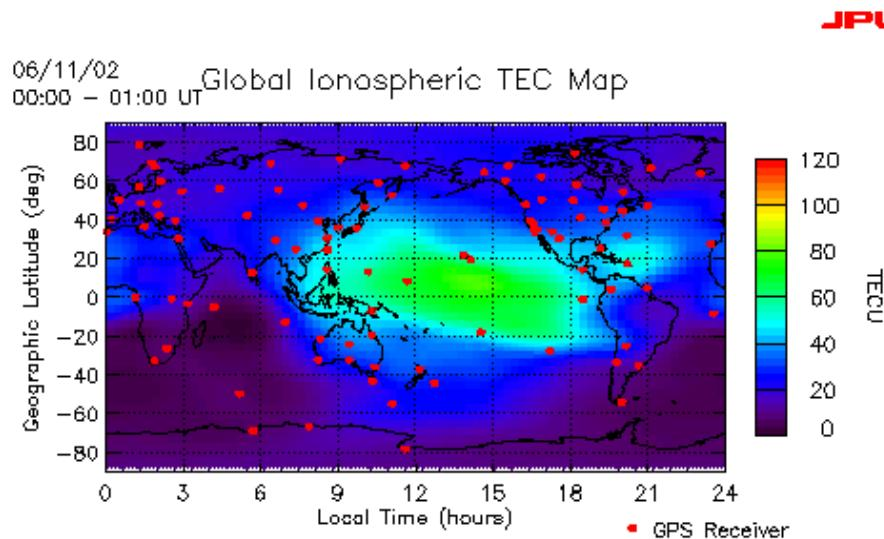
➔ In practice, the ionospheric delay is eliminated by combining the S band delay (2.3 GHz) and the X band delay (8.4 GHz).
