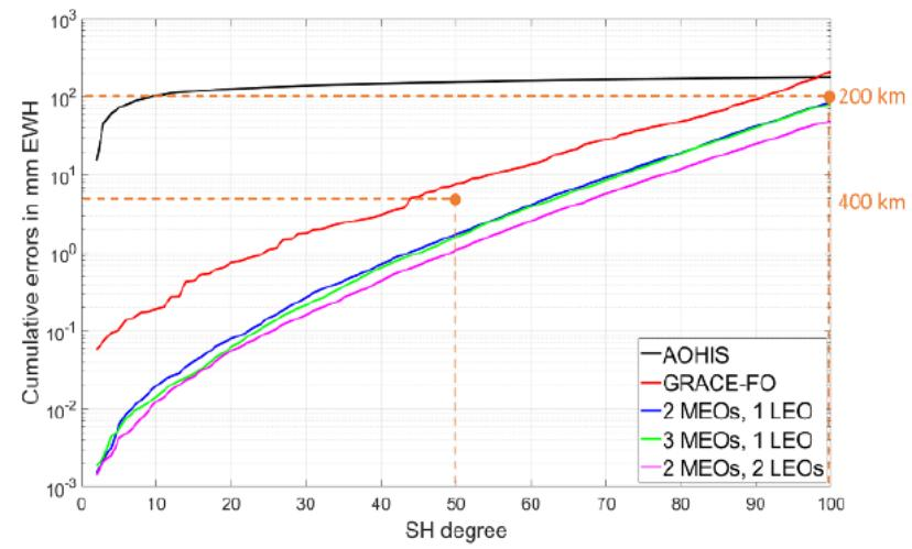
**Figure 2-5:** Degree (error) standard deviations (left) and cumulative signal/error standard deviations (right) of full AOHIS signal (black) and different mission scenarios, when including only instrument errors. The threshold science requirements for 400 km (SH degree 50) and 200 km (SH degree 100) are included in orange color.
