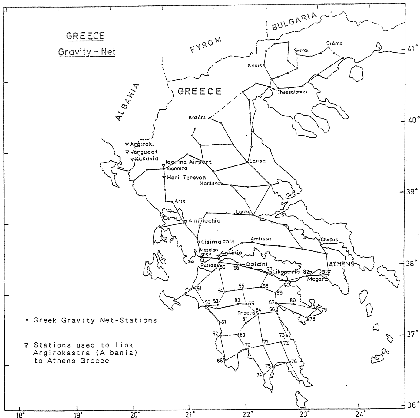
Fig. 2. 1 st order Gravity Net of Greece and the Stations used to Connect Argiokastra to Athens.
